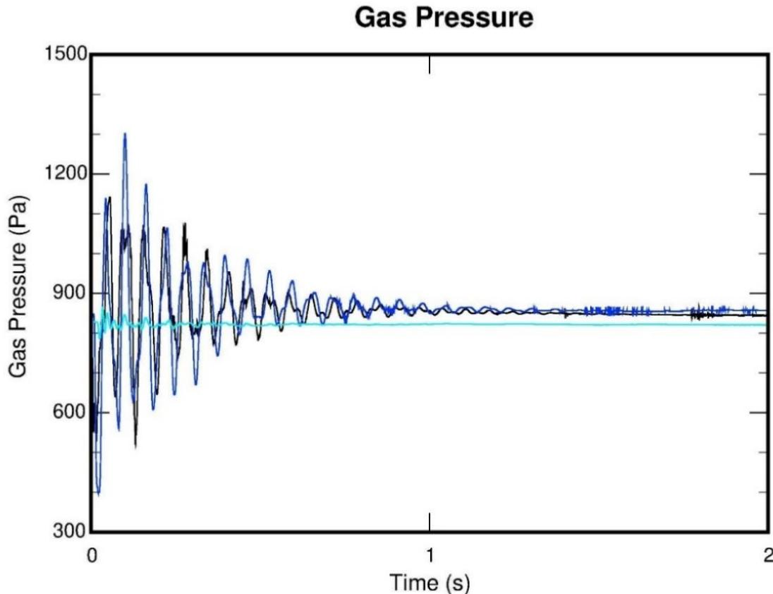
*Figure 6 - The pressure waves within the flare caused by the sudden onset of flow decay rapidly a sound free condition under no-wind conditions*
