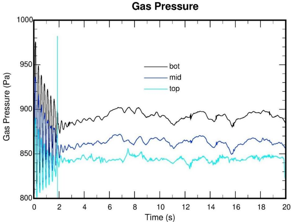
Figure 7 - The gas pressure at various elevations with a cross wind showing low amplitude persistent sound waves within the stack
