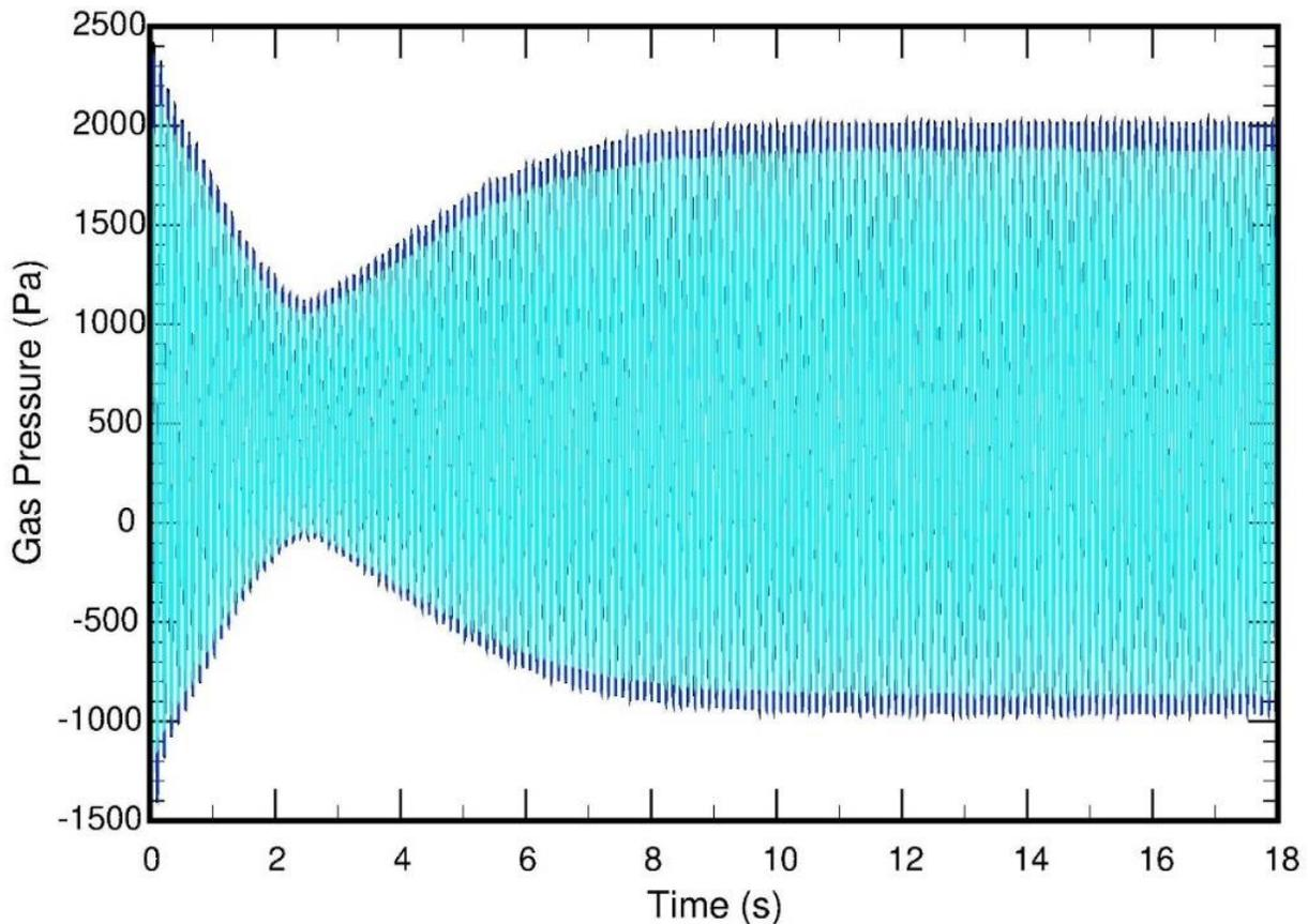
*Figure 1 – The pressure response of a simulated Sondhauss tube illustrating an initial transient that decays and later amplifies to the steady sustained oscillation [1]*
