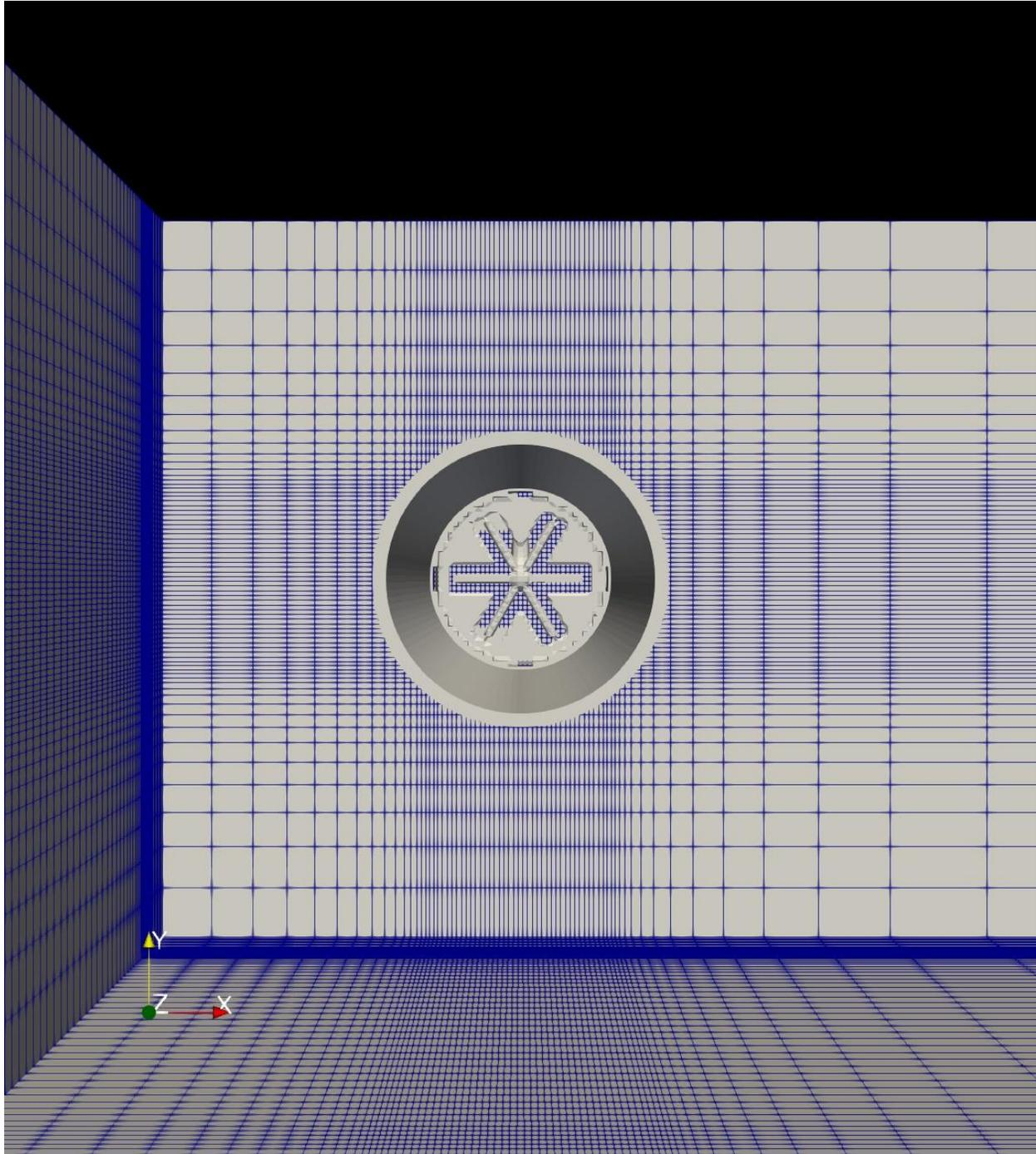
*Figure 5 – Expanded view from above showing the grid structure and some burner details*
