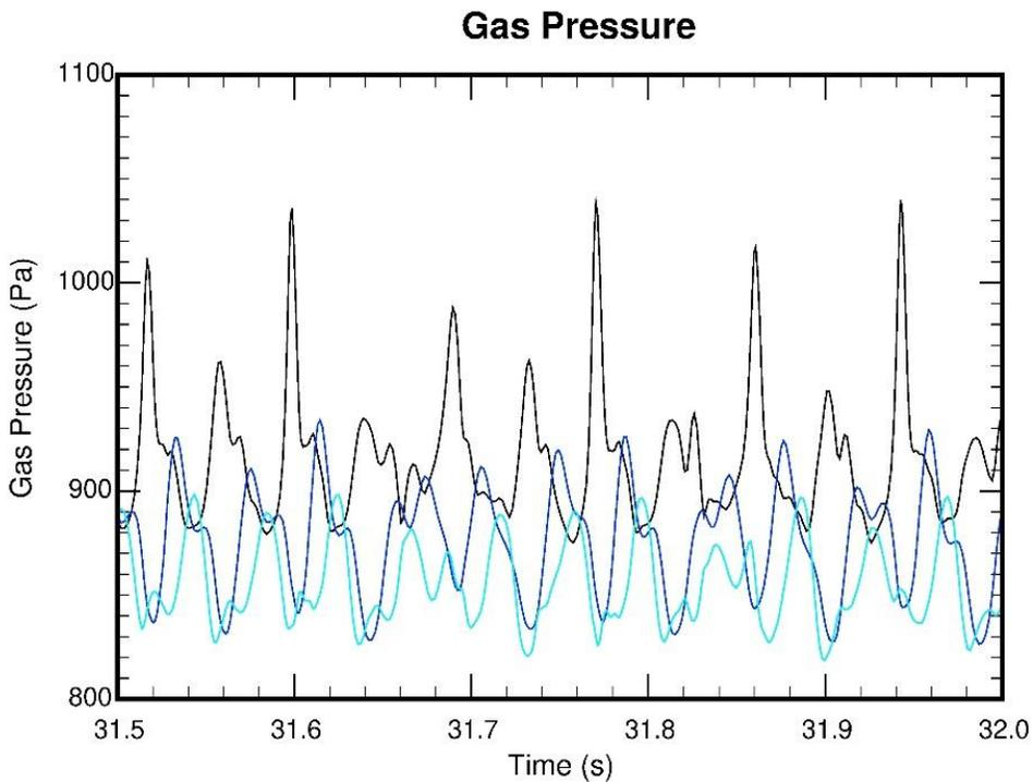
Figure 8 - Predicted pressure waves at various heights inside the operating flare considering non-uniform wind boundary conditions at the top and bottom of the flare
