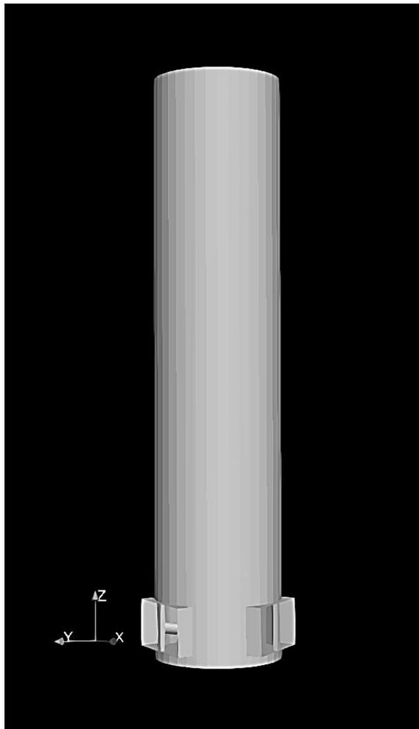
*Figure 3 – The flare used in this thermoacoustic simulation has a height of 15 meters with a diameter of 3 meters and louver openings at bottom for air inlets*
