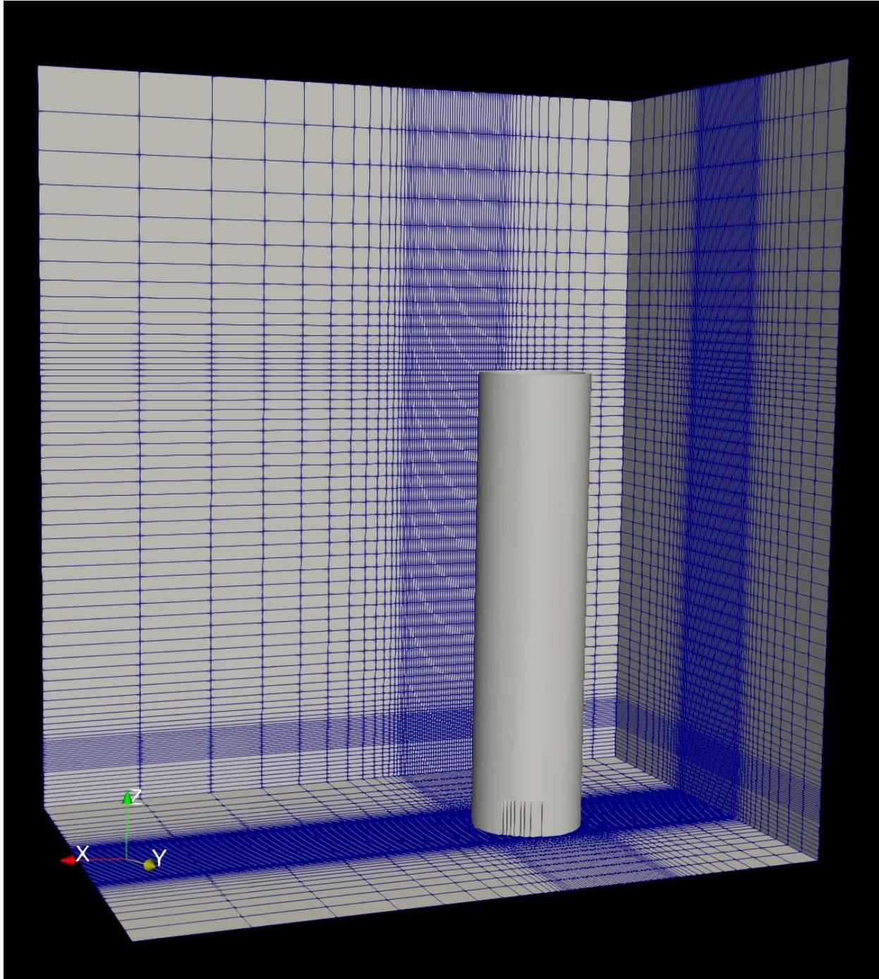
*Figure 4 - The full computational domain for the flare CFD simulation. Lines depict the grid structure*
